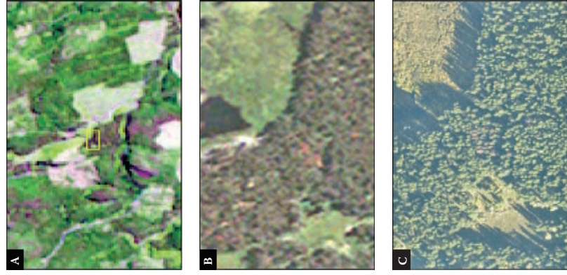
FIGURE 2.1 Illustration of differing information content for three images with differing spatial resolution located near Merritt, British Columbia, Canada. Panel A is an approximately 8 km 2 area of 30-m spatial resolution Landsat 7 ETM+ multispectral imagery (Path 46/Row 25) collected on August 11, 2001. The 0.05-km 2 focus area in Panel A is represented in Panels B and C. Panel B is 2.4-m spatial resolution QuickBird multispectral imagery collected on July 17, 2004. Panel C is a digital ortho-image with a spatial resolution of 30 cm collected on August 22, 2003.
